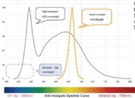
Using the phototaxis of mosquito which has the biological nature to favorite the blue violet light below 500nm, and afraid of the yellow light, that wavelength is 545-630nm and peak wavelength is 595nm, to drift away them.
