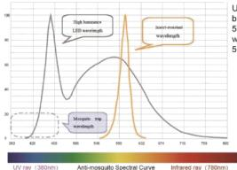
Using the phototaxis of mosquito which has the biological nature to favorite the blue violet light below 500nm, and afraid of the yellow light, that wavelength is 545-630nm and peak wavelength is 595nm, to drift away them.
